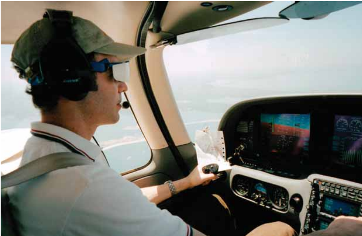
Instrument training in a Cirrus (note the back-up instruments in front of the pilot, under the PFD).
