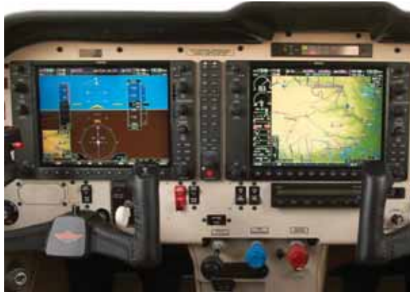
Legacy TAA Instrument panel in a Mooney Ovation 2GX.
