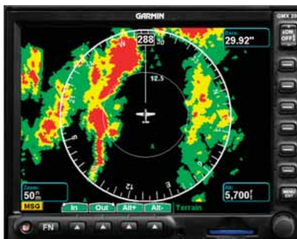
Terrain is displayed on a Garmin GMX200.
