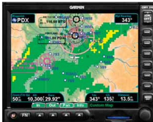
Datalinked weather is displayed on a Garmin GMX200.
