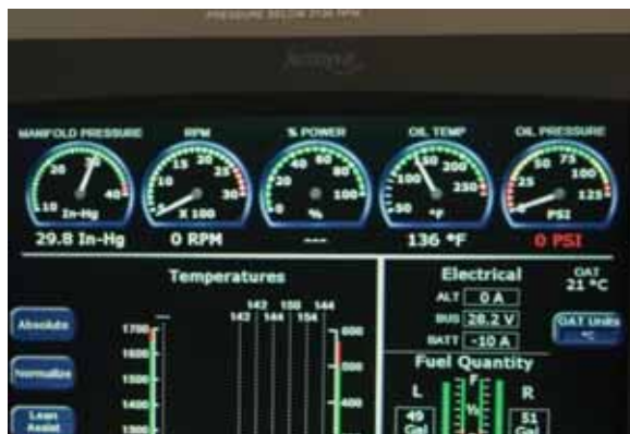
Engine monitoring display on an Avidyne Entegra system.
