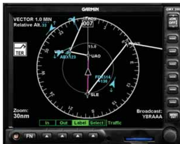
Traffic is displayed on a Garmin GMX200.
